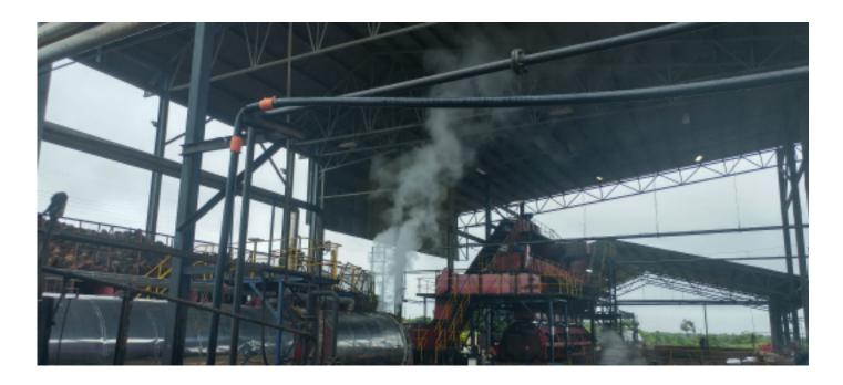
Transport of palm oil slurry at 95°C.
