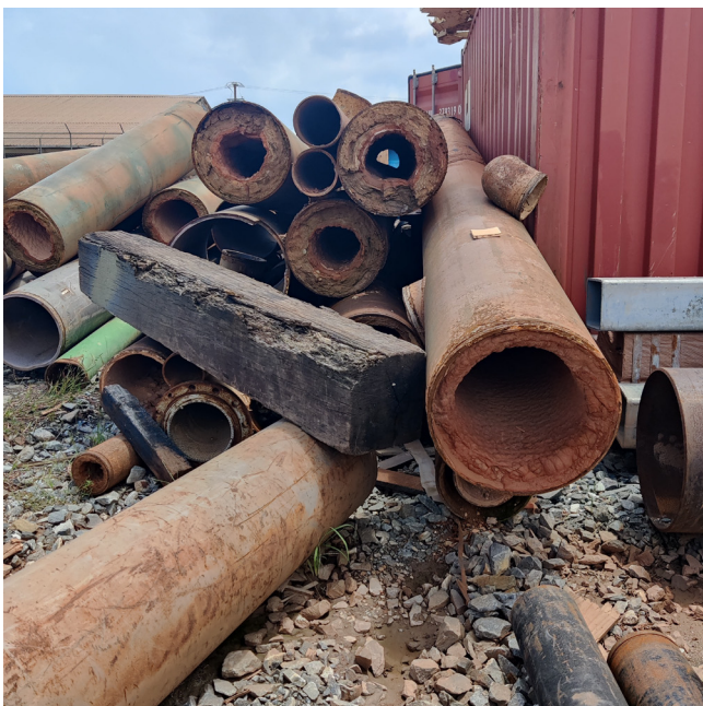
Scaled steel pipes that were replaced.
