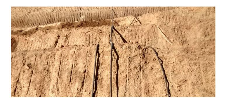
Water extraction from a middle pool to the exterior of the mine
